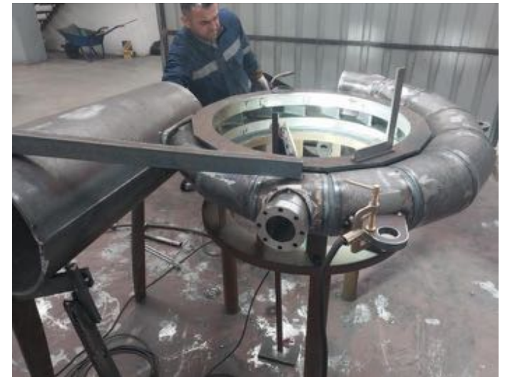
Design and build of proprietary HD turbine
